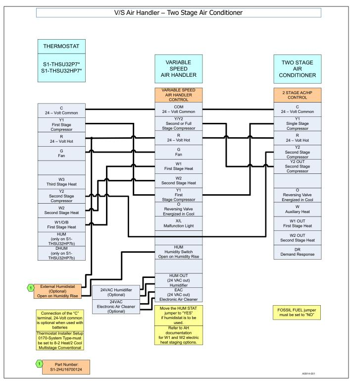
FIGURE 20: Thermostat Chart - Two Stage AC - Variable Speed Air Handler
