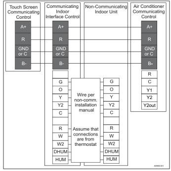
FIGURE 15: Communicating AC with Non-Communicating Air Handler or Furnace using Communicating Interface Control
