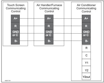
FIGURE 14: Communicating AC with Communicating Air Handler or Furnace
