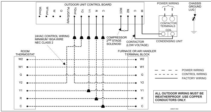
FIGURE 12: Typical 2-Stage Conventional Field Wiring - AC
