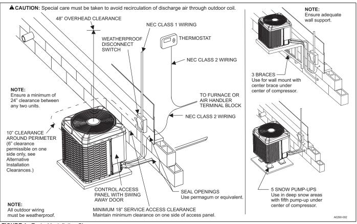
FIGURE 1: Typical Installation Clearances
