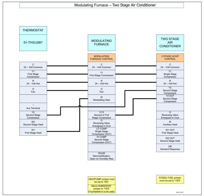
FIGURE 19: Thermostat Chart - Two Stage AC - Modulating Furnace
