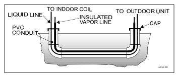
FIGURE 4: Underground Installation
