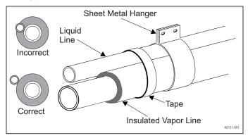
FIGURE 3: Insulation of Vapor Line
