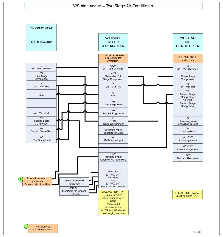
FIGURE 21: Thermostat Chart - Two Stage AC - Variable Speed Air Handler
