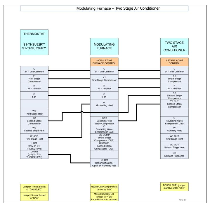
FIGURE 18: Thermostat Chart - Two Stage AC - Modulating Furnace
