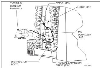
FIGURE 7: TXV Bulb and Equalizer line Installations
