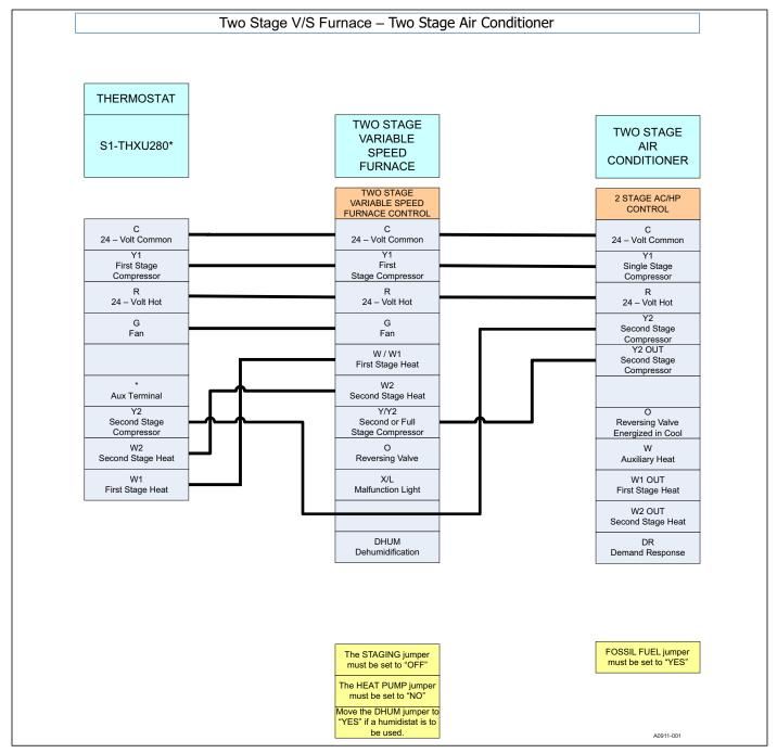
FIGURE 17: Thermostat Chart - Two Stage AC - Two Stage Furnace
