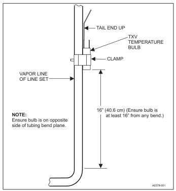
FIGURE 9: Vertical Temperature Bulb Orientation
