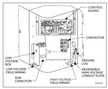
FIGURE 11: Outdoor Unit Control Box
