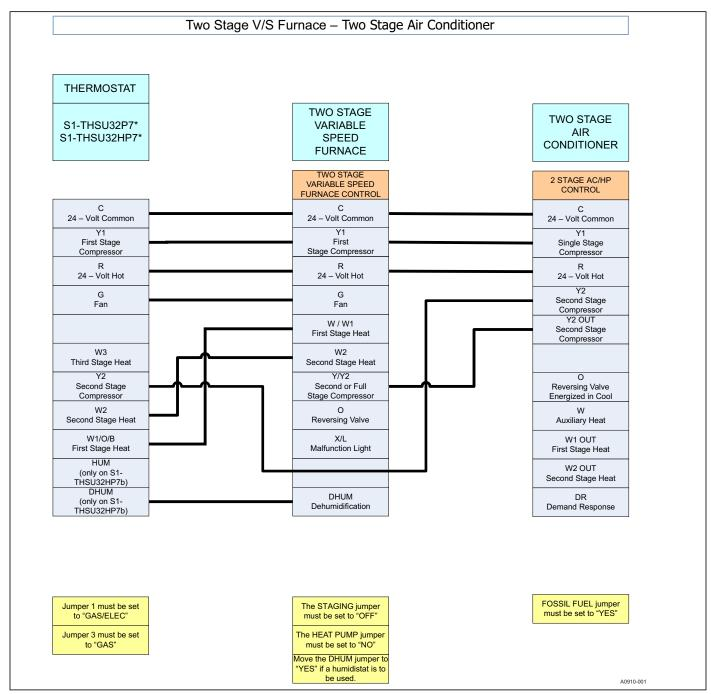
FIGURE 16: Thermostat Chart - Two Stage AC - Two Stage Furnace
