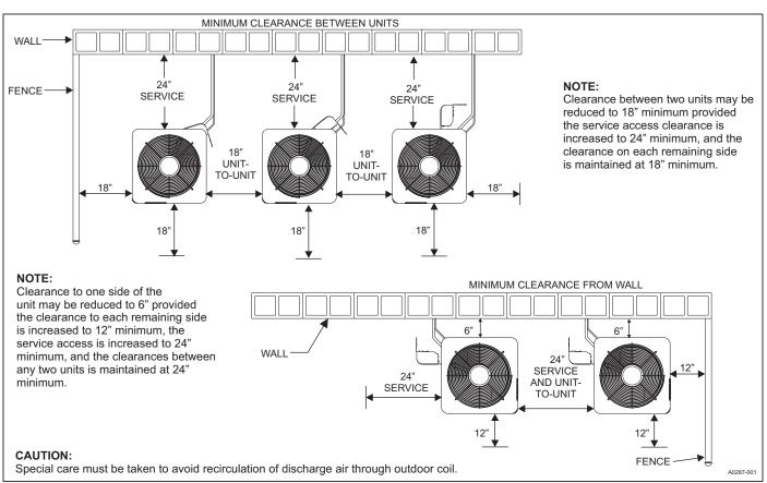
FIGURE 2: Alternative Installation Clearances
