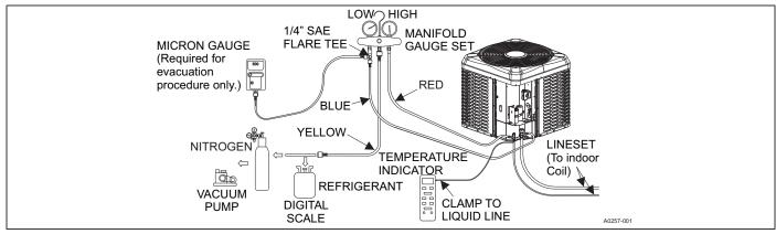
FIGURE 10: System Charging Connections
