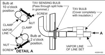
FIGURE 8: Proper Bulb Location
