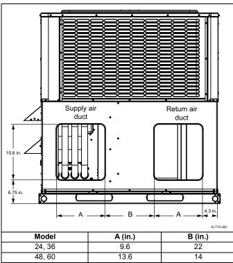
Note: See Unit dimensions and access locations for side hole sizes of electrical and gas lines.
