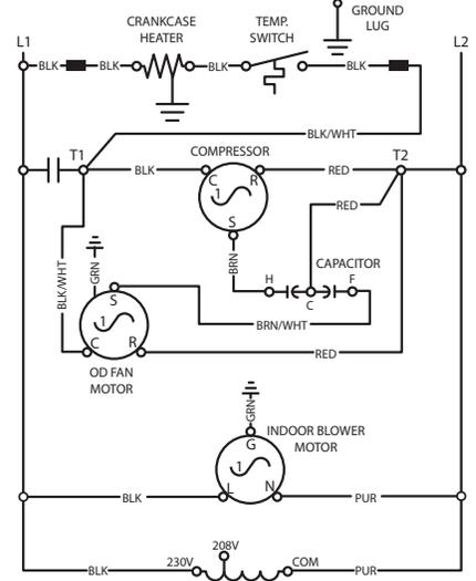
WIRING DIAGRAM FOR OPTIONAL ELECTRIC HEATER KITS:
