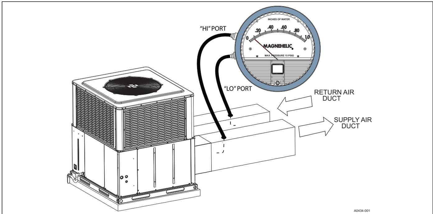
**FIGURE 11:** Measuring External Static Pressure
