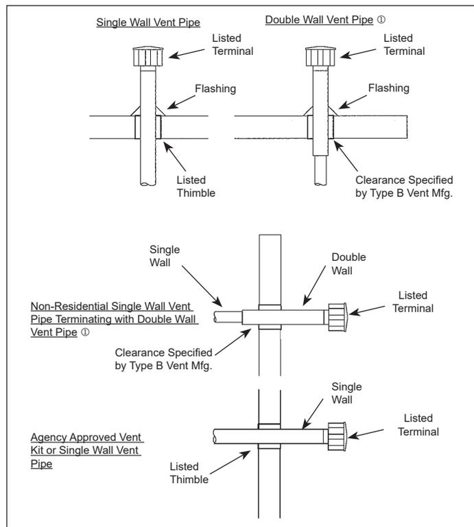
① See Instruction A10 for attaching single wall pipe to double wall pipe
