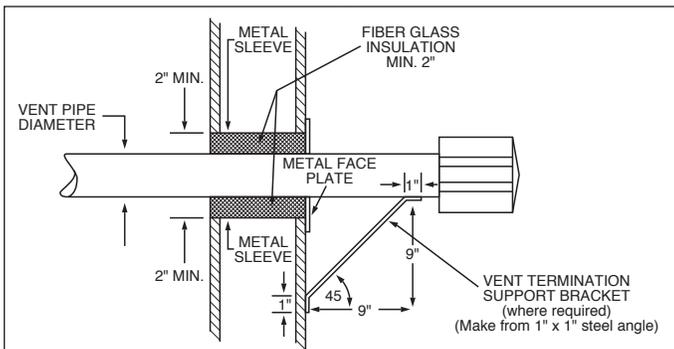
C5. When condensation may be a problem, the vent system shall not terminate over public walkways or over an area where condensate or vapor could create a nuisance or hazard or could be detrimental to the operation of regulators, relief openings, or other equipment.
