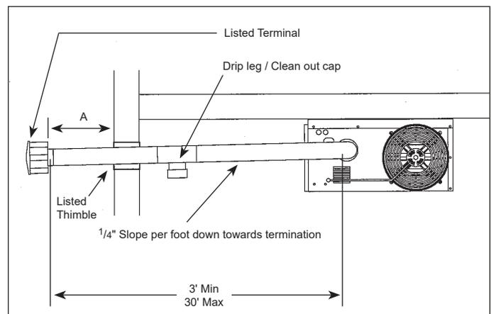
C7. When vented horizontally, maintain a 1/4" per foot rise away from the heater and place a drip leg with clean out near the unit as shown in Figure 10.2. Where local authorities have jurisdiction, a 1/4" per foot downward slope is acceptable with a drip leg and clean out near the exit of the vent as shown in Figure 10.3, or allow the condensate to drip out the end.
